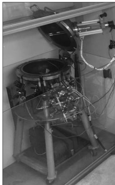
Fig. 4 Automated 20 L multi gas flammability apparatus.
