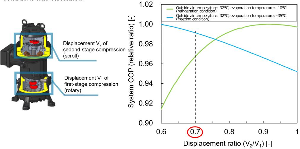
The optimum displacement ratio is different between refrigeration and freezing conditions. Considering the system COP of both conditions, the displacement ratio was determined to be  $V_2/V_1 = 0.7$ .
