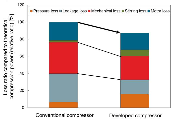
Through the reduction of mechanical loss and other factors, it was confirmed that losses could be reduced compared to conventional compressor.
