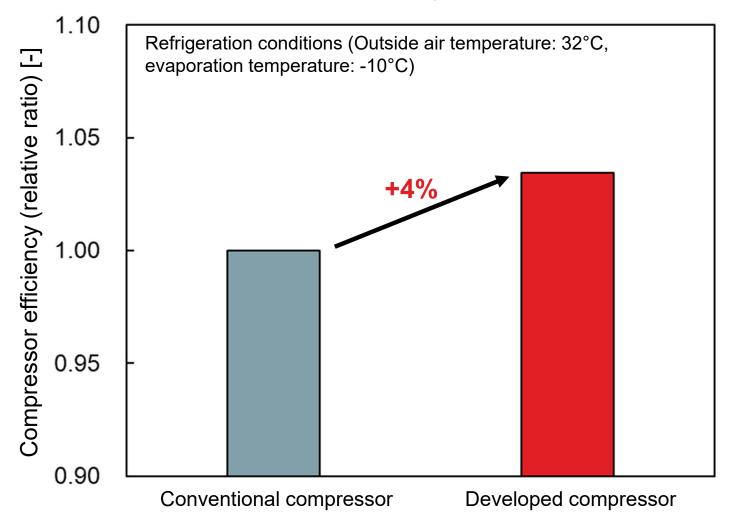
It was confirmed through measurements that the compressor efficiency (overall adiabatic efficiency) improved by 4% compared to conventional compressor.
