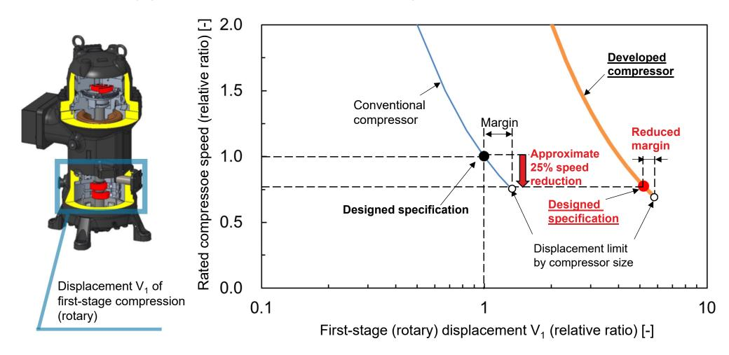
Compressor speed could be set approximately 25% lower than the conventional compressor by reducing the margin of displacement limit by compressor size.
