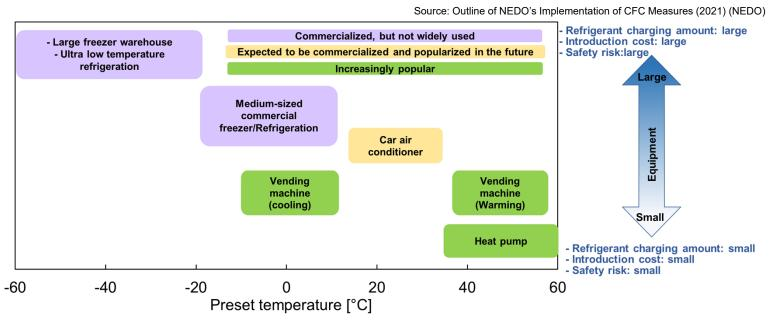
Although CO<sub>2</sub> is mainly used for refrigeration, freezer and heat pump, product development for further popularization is desired. Our company put two-stage compressor for CO<sub>2</sub> refrigerant on the market in 2011.
