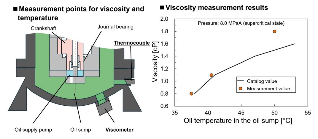
At around 50°C oil temperature, the difference between the measured values and the catalog values was confirmed.
